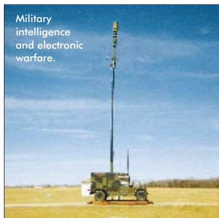
Elevated cameras, communications antennas and emergency lighting on mobile command post vehicles.
